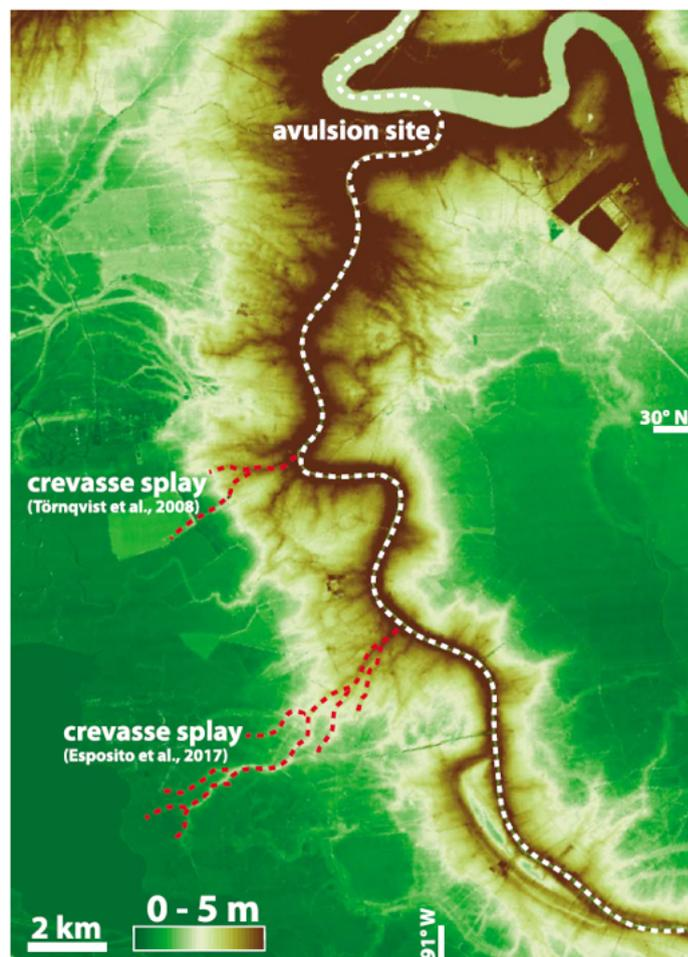
FIGURE 2.4: LIDAR image of crevasse splay and avulsion caused by natural levee breaches. From Nienhuis et al. [2018].
